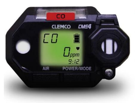
The CMS-4 attaches inside the helmets of supplied-air respirators. which enables blast operators to self-monitor their CO exposure. It triggers audible, visual, and vibratory alarms if CO is detected in concentrations of at least 10 ppm.
