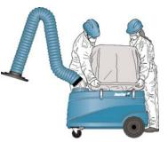
Release filter cover clips and lift off the filter cover.
