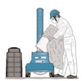
Release filter cover clips and lift off the filter cover.
